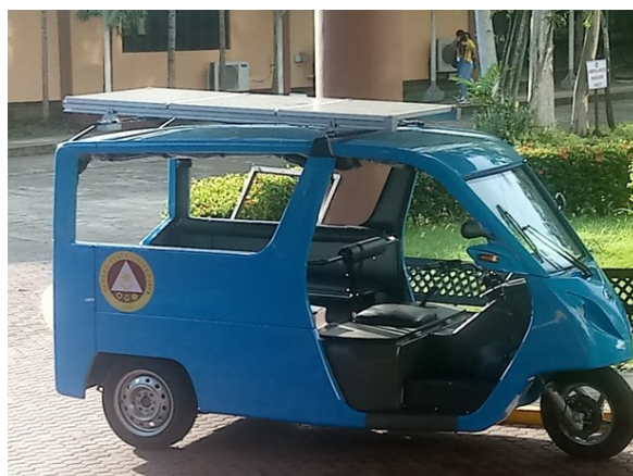
Figure 2. 68VM e-trike after installation of the solar charger
