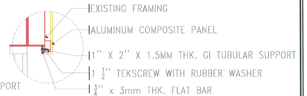
BLOW UP DETAIL D SCALE 1:10MTS
